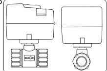
Actuator has the function of manual adjustment which is convenient for on-site operation.
